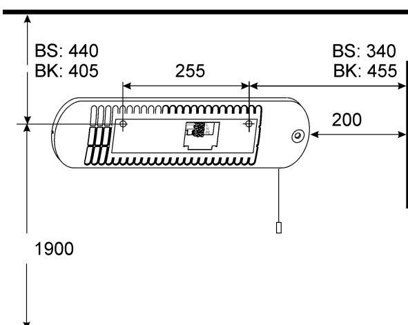
It is not permissible to install the device vertically or on the ceiling.
