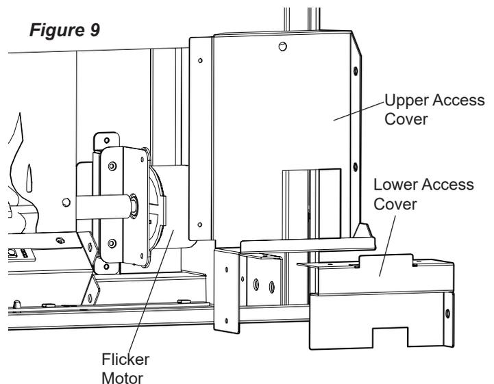
**⚠ CAUTION:** When removing and replacing the flicker motor try to keep any slight bending of the flicker rod minimal so as to not damage it. If flicker rod is damaged, it should be replaced to ensure proper operation.
