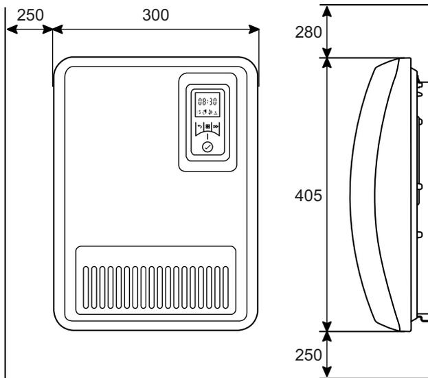
The minimum clearances must be observed. In addition, a clearance of 750 mm is to be maintained in front of the unit.
